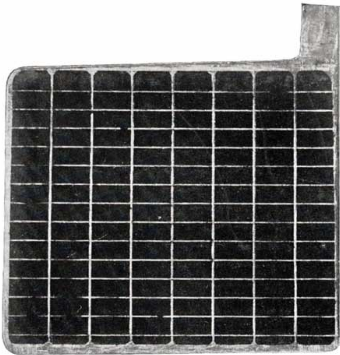
Fig. 7. Formed Plate, Ready to Be Burned to Plate Connecting Strap
