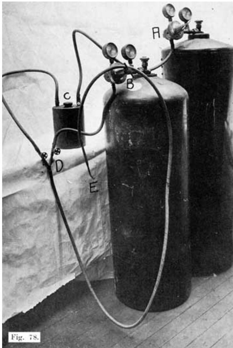
Fig. 78. Hydrogen-Oxygen Lead Burning Outfit. A and B are Regulating Valves. C is the Safety Flash Back Tank. D is the Mixing Valve. E is the Burning Tip.
